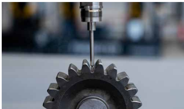
Fig. 1: UCI testing with SONODUR
